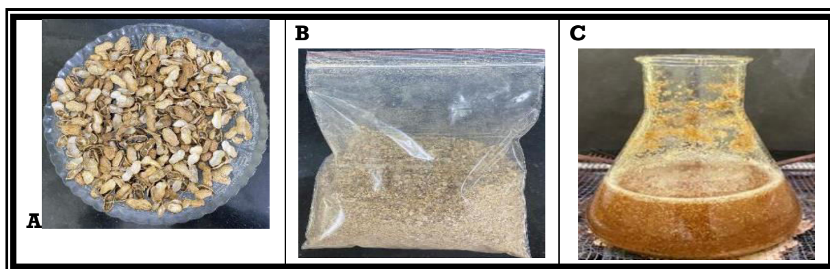
Figure-1(A-C): Figures describing (A) Dried peanut shell, (B) Powdered peanut shell, (C) Boiled with dis.H 2 O
