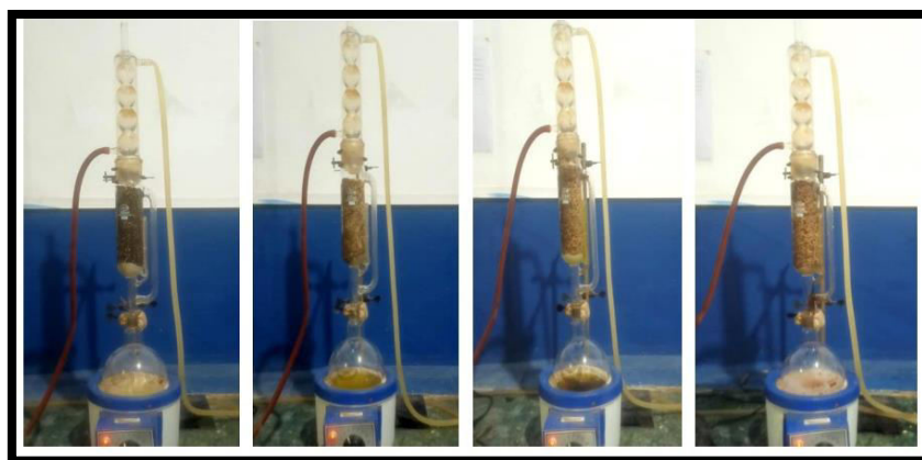
Figure1: Soxhlet Extraction of Ziziphus nummularia using Petroleum Ether, Ethyl acetate, Methanol and Aqueous solvents respectively.
