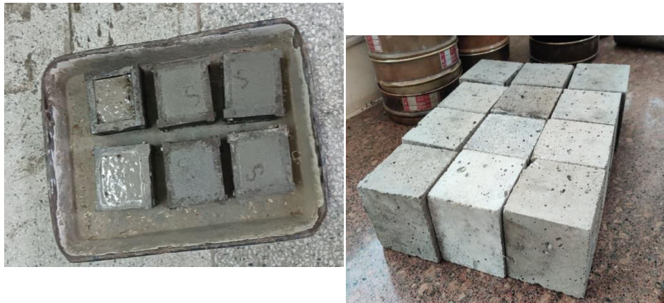
Photograph 2: Specimens casting and demolding
