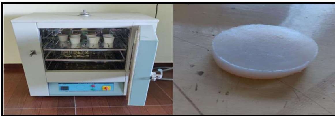
Figure 2. (a) Hot air oven used for curing; (b) Hardened geopolymers resin disc.
