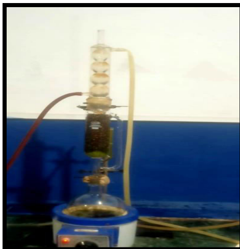
Figure 5: Soxletation of Artemisia vulgaris with Hydro alcoholic solvent
